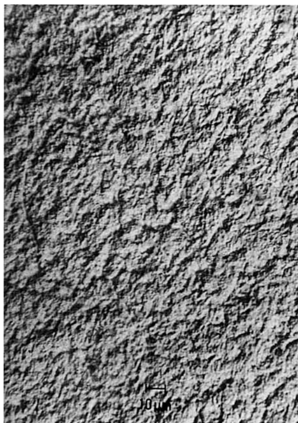
Figure 1 LLDPE 7, Blocking Force = 16.0 g. Blown films fabricated with 0.76 mm (30 mil) die gap.
