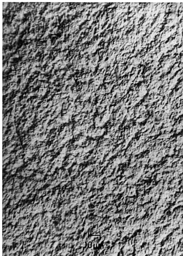
Figure 2 LLDPE 8, Blocking Force = 24.3 g. Blown films fabricated with 0.76 mm (30 mil) die gap.
